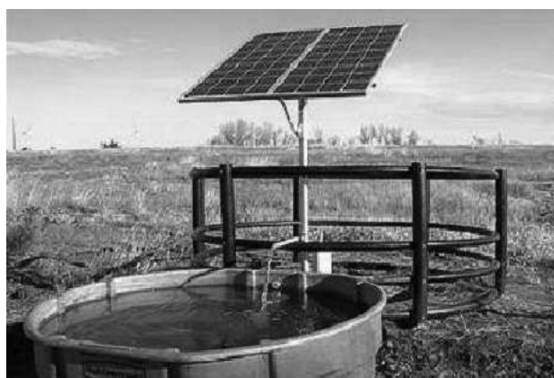
Fig.2. Photovoltaic pumps with solar array
